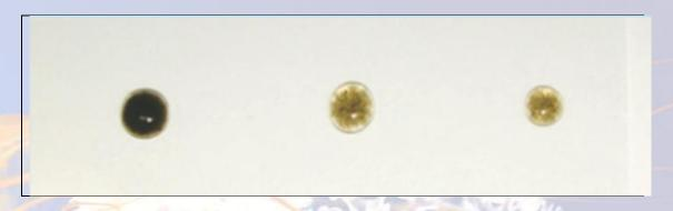
Fig. 5. Treated settled sludge samples from the bottom of a lagoon appear darker than untreated settled sludge and mixed liquor suspended solids (MLSS).
